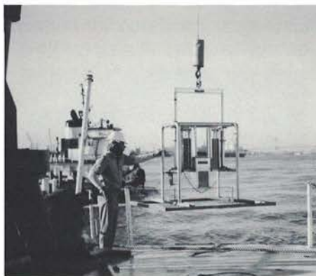
Left: Submersible camera apparatus is lowered into the Delaware River from the deck of the OSV Peter W. Anderson as part of the sediment oxygen demand study.
