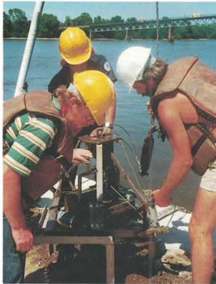
Personnel from the U.S. Environmental Protection Agency prepare to take a sediment sample from the Delaware estuary for use in studies on sediment oxygen demand and toxics. (Photo courtesy Richard C. Albert)
