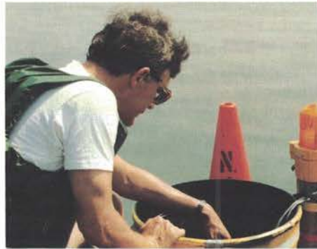
Dick Albert, supervising engineer in the Commission's Water Quality and Planning Analysis Section, inspects a Minimonitor inside a trash can on one of the platforms. The trash barrels housed the delicate monitoring equipment which received and recorded signals from submerged sensors. Parameters measured included water temperature, dissolved oxygen, conductivity and pH. (Photo by Warren Huff)
