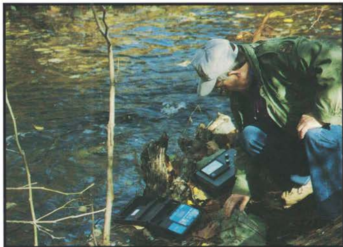
Richard Albert, DRBC supervising engineer, checks readings on a conductivity meter and a dissolved oxygen meter while doing water quality sampling work on Sawkill Creek near Milford, Pa. (Photo by Elizabeth Johnson)
