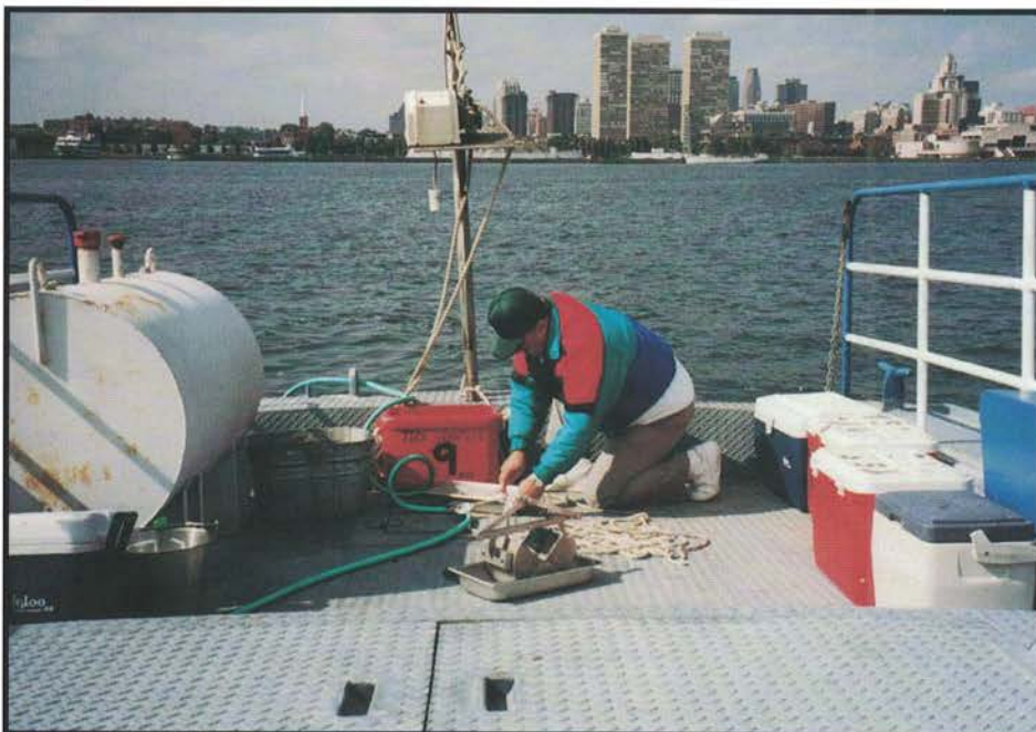
Ron Rulon, a sanitary engineer in the Commission's water quality implementation section, cleans sediment sampling equipment onboard the "Delaware." A device with a clamshell bucket is lowered to the river bottom where it scoops up sediment to be analyzed for toxic metals and organic chemicals. Philadelphia is in the background. (Photo by Tom Fikslin)
