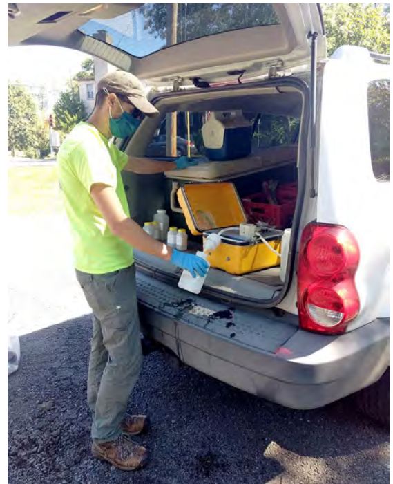
Frequent water quality data collection continued in 2020 for this project once laboratories opened and safety protocols were approved for implementation. DRBC Aquatic Biologist Jake Bransky preserves a sample for analysis collected from the Falls Bridge, Schuylkill River. Photo by DRBC.
