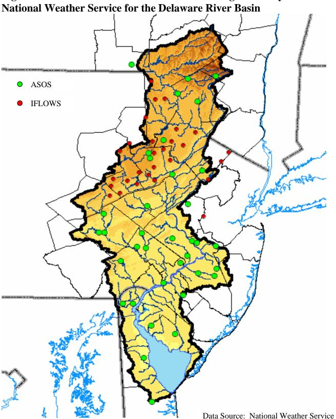
Figure A-2: Location of ASOS and IFLOWS Gages Used by the National Weather Service for the Delaware River Basin
