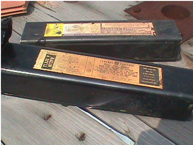
Intact non-PCB ballasts from 8-foot lamps.
