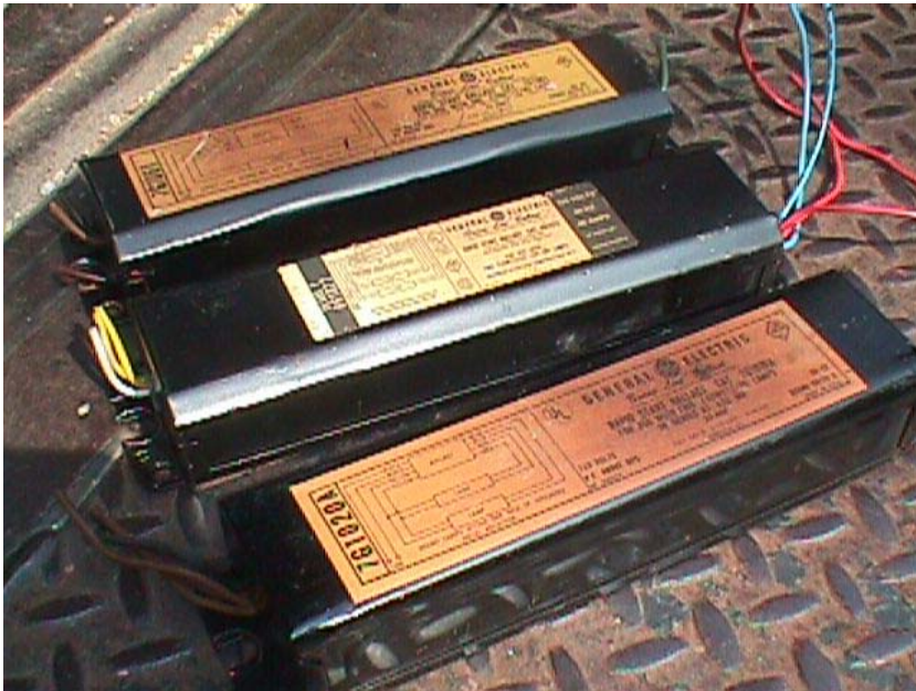
PCB lamp ballasts
