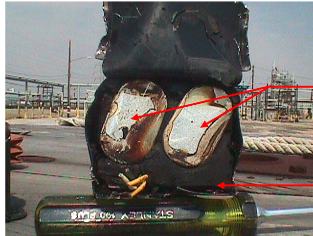
Metal end removed shows bottom of two wet-capacitors (liquid filled) and surround potting material.
