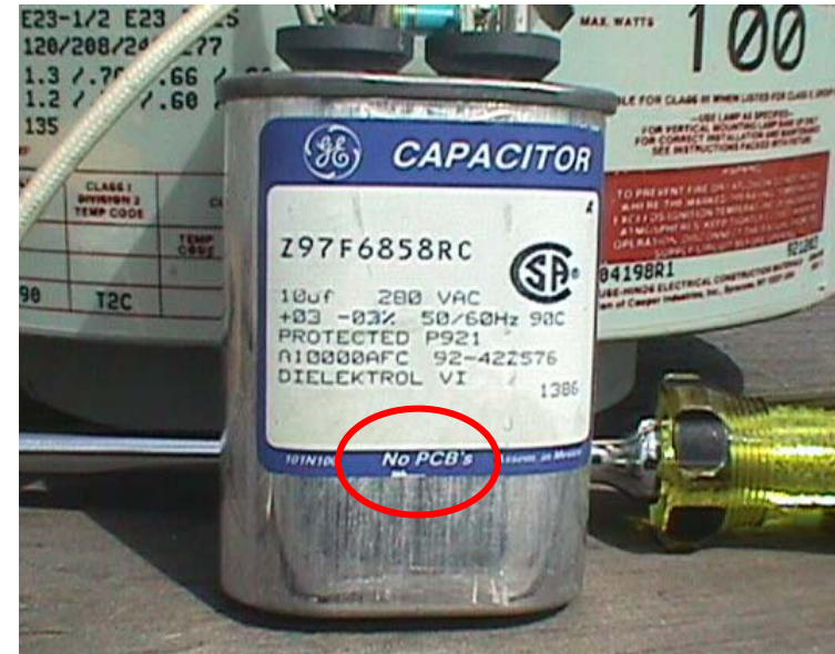
You must remove and examine the small capacitor. Note: "No PCBs" on label.
