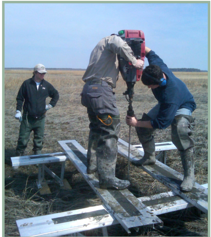
Fig. 5.31. Scientists from the Academy of Natural Sciences, Partnership for the Delaware Estuary, and Rutgers University installing a surface elevation table in a salt marsh in the Dennis Creek watershed, New Jersey, in March 2011 as part of a new sub-regional monitoring initiative targeting tidal wetlands: the Mid-Atlantic Coastal Wetland Assessment
