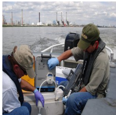
DRBC staff collects a filtered sample during a July 2012 special copper survey in the Delaware Estuary.
