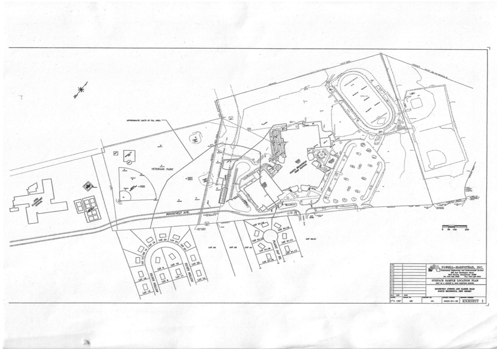
Figure 3: Approximate boundary of the buried waste material area encompassing the North Brunswick Township High School (NBTHS) , PSE&G easement, and Veteran’s Park properties. New building addition to the NBTHS is depicted on the southwest corner of the high school (formerly “The Oval”).
