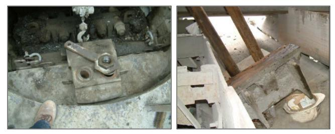
Photo 2 Top of Jaw Crusher Showing Toggle Block Retaining Clamp, Nut, and Wrench
