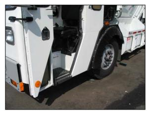
Photo 2 Entry Step to Recycling Truck
