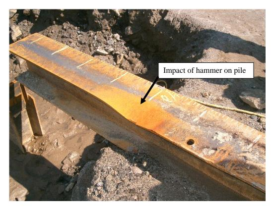
Figure 4: Pile as it rested after crushing victim. Note the muddy conditions.
