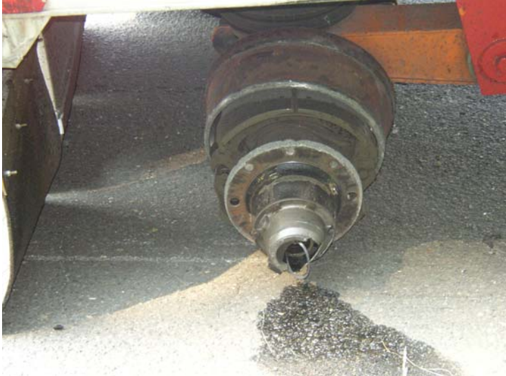
Figure 4: Axle of trailer from which the wheel separated
