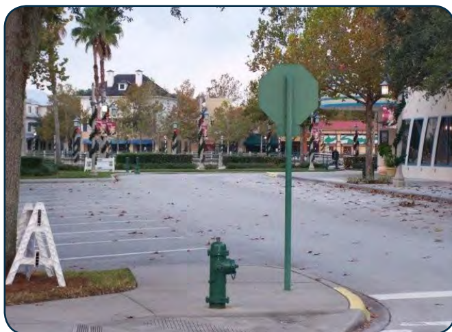
Although a new town, Celebration, Florida paints the back sides of its signs to blend these features with the landscape. (Courtesy of Strong Towns).
