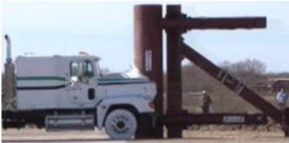
(a) Engine impact on pier during field testing
