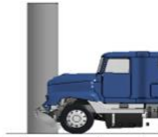
(b) Engine impact on pier in LS-DYNA
