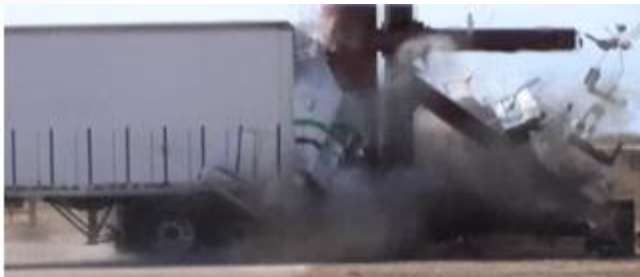
(a) Trailer impact on pier during field testing
