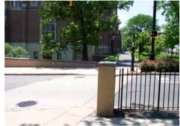
Decorative iron fencing guides pedestrians to crosswalks, deterring jaywalking.
