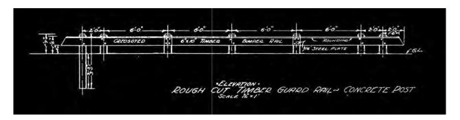
Elevation of rough cut timber guard rail taken from the original design drawings for the Palisades Interstate
