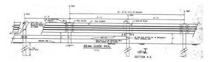
W Beam guiderail section taken from the NJDOT design drawings for the Palisades Interstate Parkway
