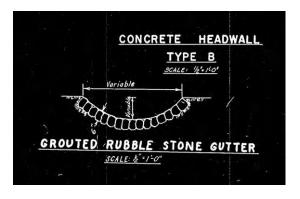
Stone gutter detail taken from the original design drawings for Henry Hudson Drive
