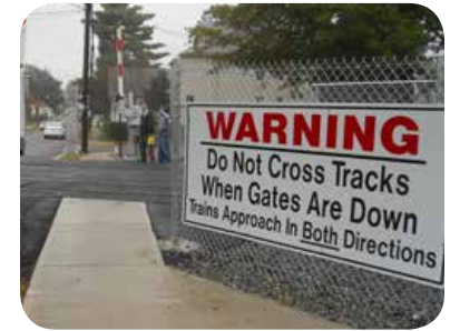
Example of a nonstandard sign in Garfield, NJ. Photo also shows how the sidewalk leads pedestrians up to the designated, desired crossing point. Image: The RBA Group
