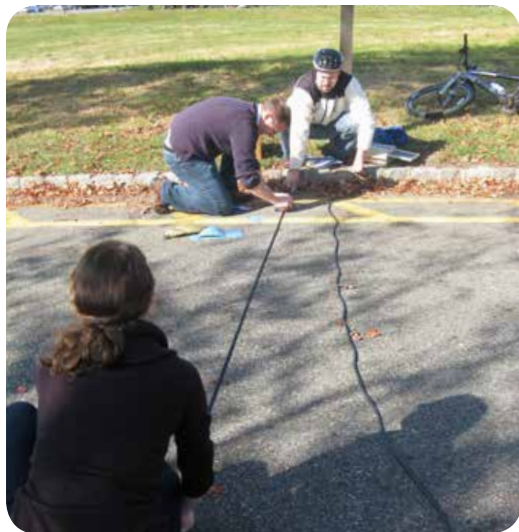
Pneumatic tubes can record speeds and volumes. Image: The RBA Group
