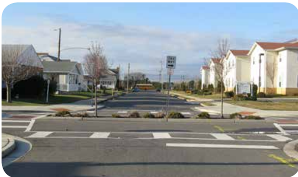
This landscaped median along Haven Avenue in Ocean City, NJ allows right turns only for motor vehicles. Image: The RBA Group
