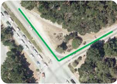
This high-speed ramp has been replaced with a 90-degree intersection. Image: California Department of Transportation
