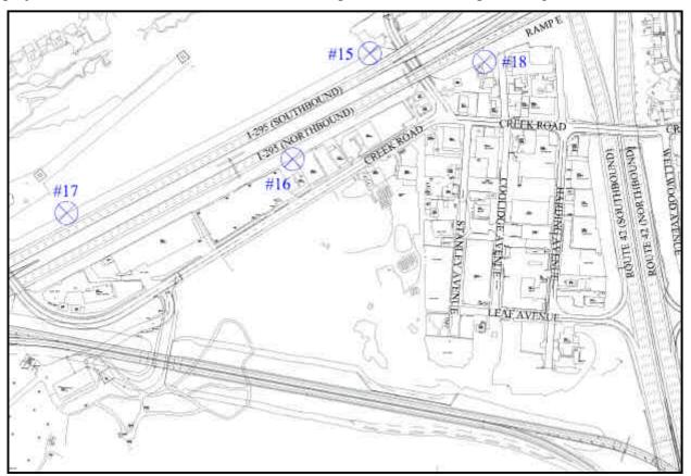
Receptor #15 and Receptor #17 are located along the I-295 southbound right-of-way line, representing the neighborhoods near Essex Avenue, Creek Road and Booth Drive. Receptor #16 and Receptor #18 are located along the I-295 northbound right-of-way line, representing the neighborhoods near Creek Road, south of the Interchange.
