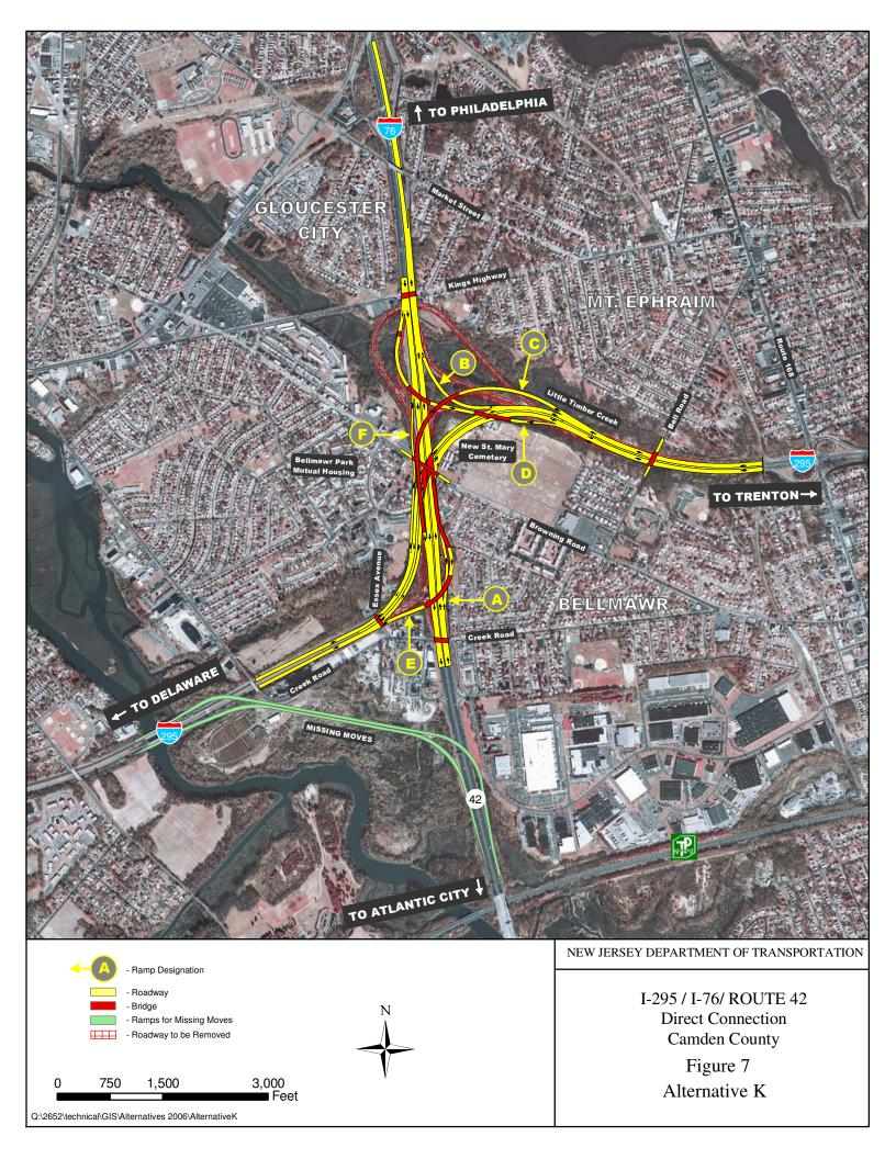
Northbound I-295 traffic heading north on I-76 utilizes Ramp E which follows essentially the same alignment as it does now.
