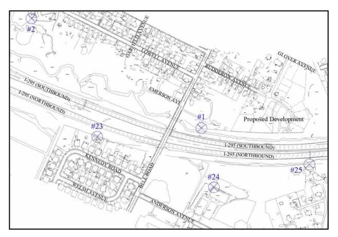
Receptor #1 is located along the I-295 southbound right-of-way line, representing the neighborhoods near Bell Road as well as Lowell, Emerson and Rudderow Avenues. Receptor #23 and Receptor #25 are located along the I-295 northbound right-of-way line, representing the neighborhoods near Bell Road, Kennedy Road and Anderson Avenue. Receptor #2 represents the Shining Star Park, while Receptor #24 represents the Scott E. Mueller Park.
