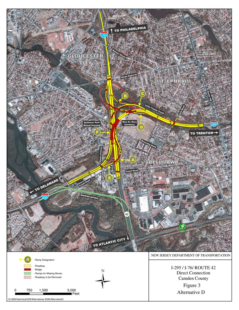
Ramp D is the move from I-76 southbound to I-295 northbound. Ramp D exits I-76 in much the same way that it does now. The Ramp D alignment crosses over I-76, over Ramp C, and under I-295 before merging with I-295 northbound south of Bell Road.
