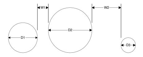
FHWA Culvert Inspection Manual - July 1986 Section 3-1.1 e. - Multiple Barrels
