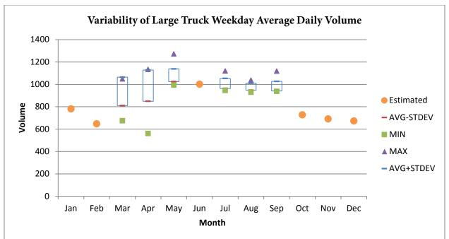
Figure 0-64. Variability of Large Truck Volume at Northbound I-95, MP 6.3 (2010)
