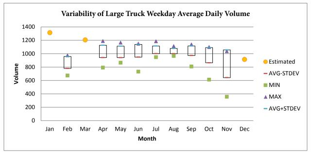
Figure A-61. Variability of Large Truck Volume at Northbound I-95, MP 6.3 (2009)
