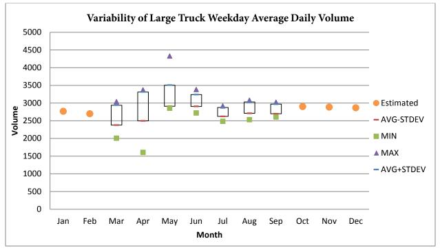
Figure A-108. Variability of Large Truck Volume at Northbound I-295, MP 39.6 (2010)
