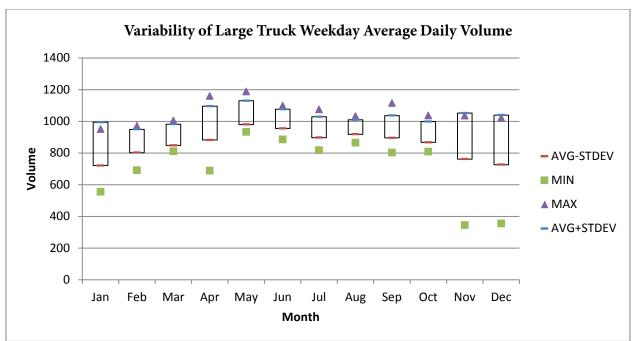
Figure A-55. Variability of Large Truck Volume at Northbound I-95, MP 1.2 (2009)
