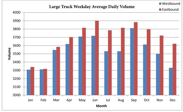
Figure A-30. Annual Profile of Large Truck Volume at I-80, MP 8.3 (2011)
