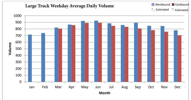
Figure A-51. Annual Profile of Large Truck Volume at I-195, MP 10.2 (2011)
