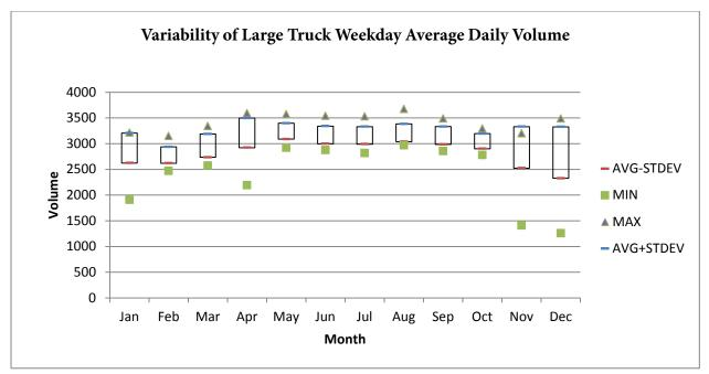
Figure A-105. Variability of Large Truck Volume at Northbound I-295, MP 39.6 (2009)
