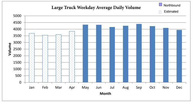
Figure A-69. Annual Profile of Large Truck Volume at Northbound I-287 MP 31.7(2009)
