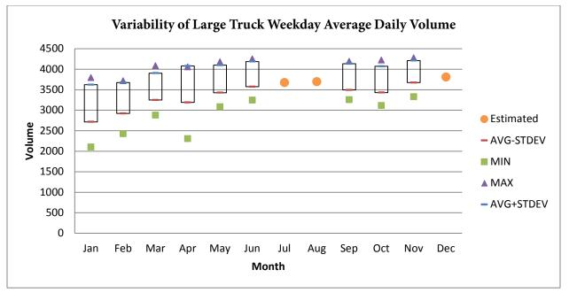
Figure A-87. Variability of Large Truck Volume at Northobund I-287 MP 61.7 (2011)
