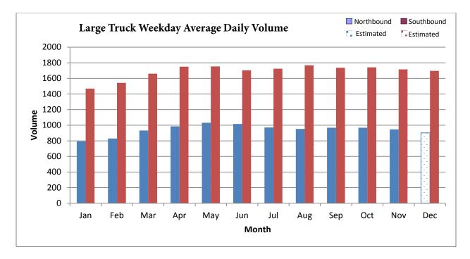
Figure A-66. Annual Profile of Large Truck Volume at I-95, MP 6.3 (2011)
