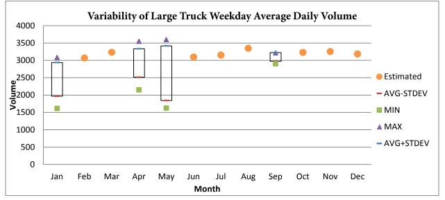
Figure A-95. Variability of Large Truck Volume at Northbound I-295, MP 35.7(2010)
