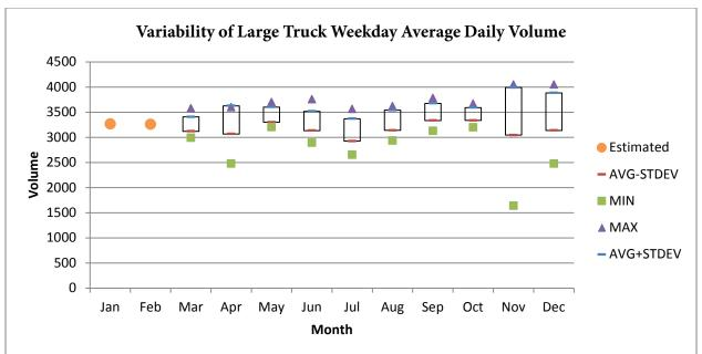
Figure A-100. Variability of Large Truck Volume at Northbound I-295, MP 35.7(2011)
