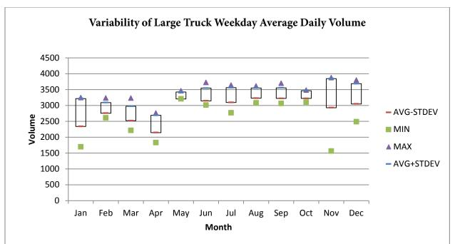
Figure A-113. Variability of Large Truck Volume at Northbound I-295, MP 39.6 (2011)
