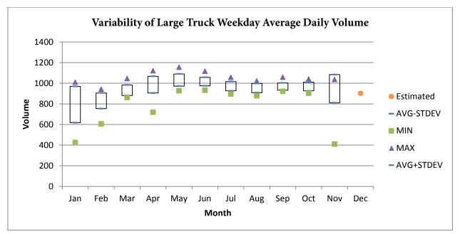
Figure A-67. Variability of Large Truck Volume at Northbound I-95, MP 6.3 (2011)
