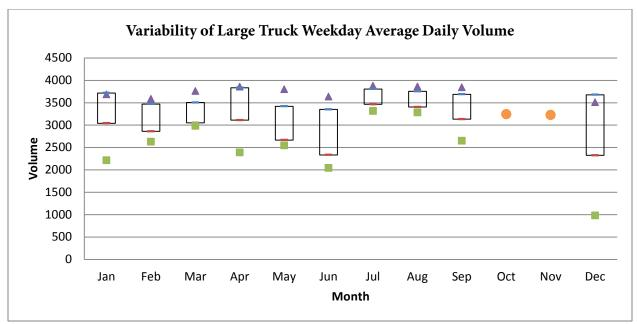
Figure A-92. Variability of Large Truck Volume at Northbound I-295 MP 35.7(2009)
