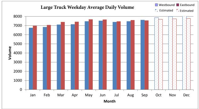
Figure A-14. Annual Profile of Large Truck Volume at I-78, MP 14.5 (2010)
