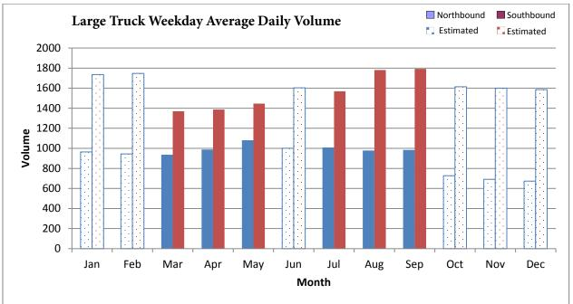
**Figure 0-63.** Annual Profile of Large Truck Volume at I-95, MP 6.3 (2010)
