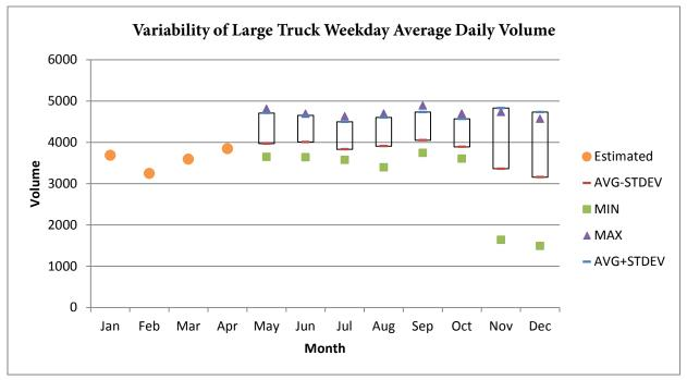
Figure A-70. Variability of Large Truck Volume at Northbound I-287, MP 31.7 (2009)
