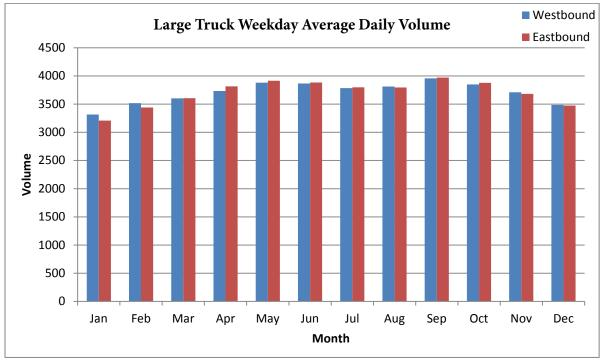
Figure A-22. Annual Profile of Large Truck Volume at I-80, MP 8.3 (2009)
