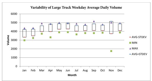
Figure A-75. Variability of Large Truck Volume at Northbound I-287, MP 31.7(2011)
